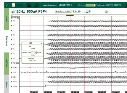
Figure 4a: Sinusoidal stimulation 20 Hz/500  $\mu$ A<sub>pp</sub> at C3, C4. Amplitudes increases slowly at the stimulation start.
