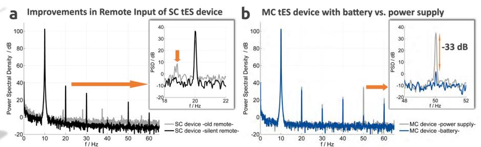
Use battery-operated tES devices with best noise profiles.
